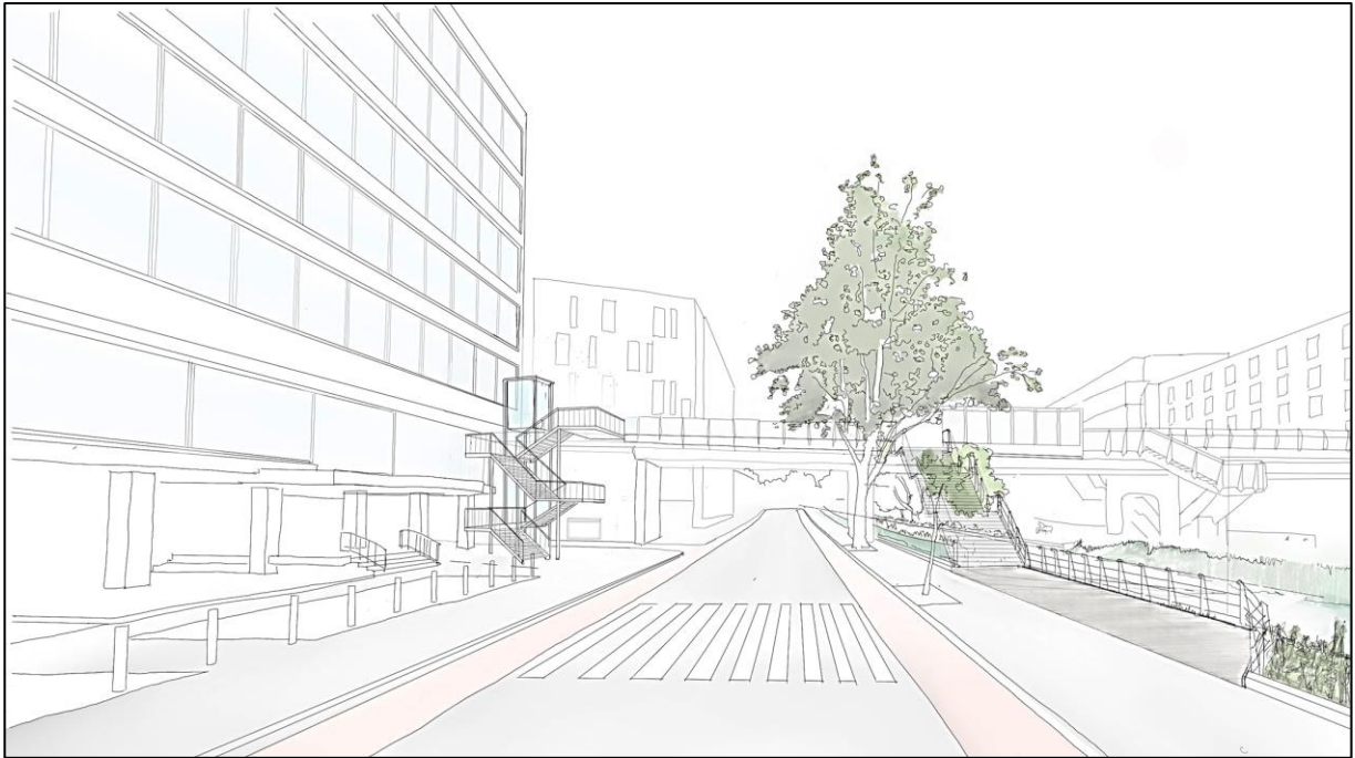
Figure 2.2: Option 2 – Pedestrian Crossing on Grand Parade leading to walkway deck extended out along canal bank and stairs to Luas platform on northside of Grand Parade. PRM lift placed on south side of Grand Parade adjacent to the Carroll's building. (note stairs on south side adjacent to the Carroll's building would not be included in this option).
